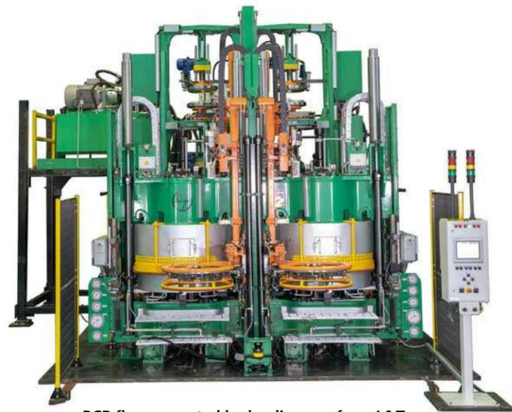
PCR floor-mounted hydraulic press from L&T
